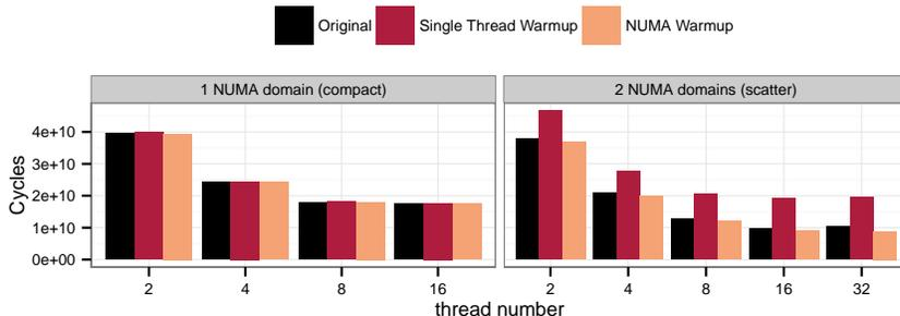
**Fig. 4.** Prediction accuracy of a single-threaded warmup versus a NUMA aware warmup on BT `xsolve`. Only a NUMA aware warmup is able to predict this region execution time on a multi NUMA domain configuration.
