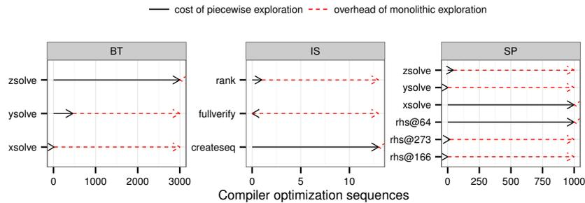
**Fig. 12.** Compiler sequences required to get a speedup over  $1.04\times$  per region. CERE evaluates the sequences in the same order for all the regions. Exploring regions separately is cheaper because we stop tuning a region as soon as the speedup is reached.
