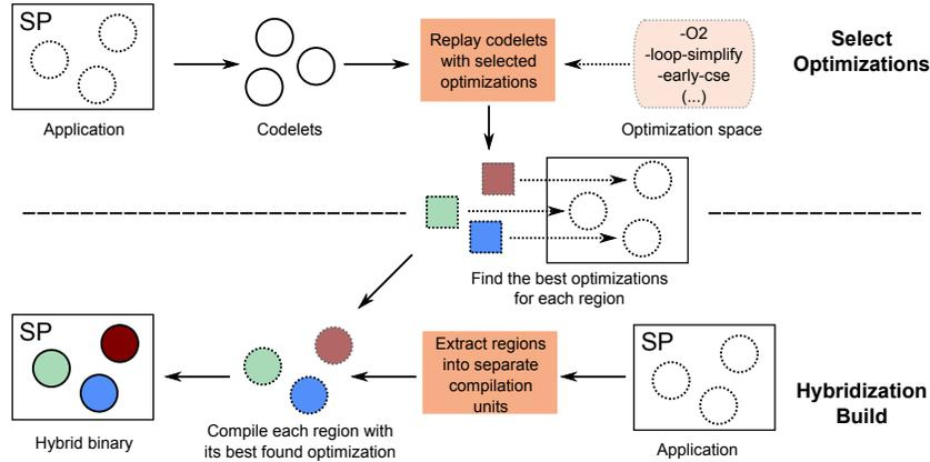
**Fig. 10.** Hybrid compilation process. Through codelets, CERE finds the best compiler sequence for each region. Then, each region is compiled with its best compiler sequence in the original application.
