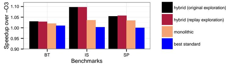
**Fig. 13.** Speedups over `-O3`. We only observe speedups from the iterative search over BT, SP, and IS. Best standard is the more efficient default optimization (either `-O1`, `-O2`, or `-O3`). Monolithic is best whole program sequence optimization. Hybrid binaries are build upon optimizations found either with codelets or with original application runs.
