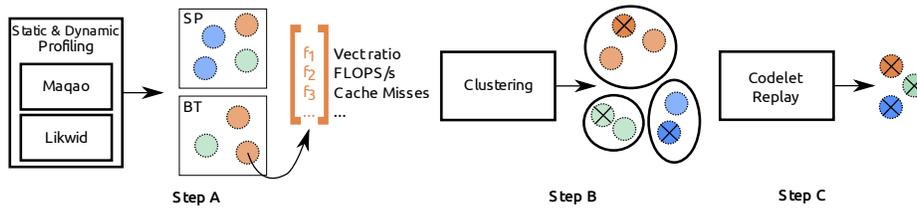
**Fig. 9.** Clustering codelets for fast compiler optimization tuning. Step A: perform static and dynamic analysis to capture codelets metrics vectors. Step B: by using the proximity between metrics vectors, CERE clusters similar codelets and selects one representative per cluster. Step C: CERE extracts and replays the representatives as standalone codelets.
