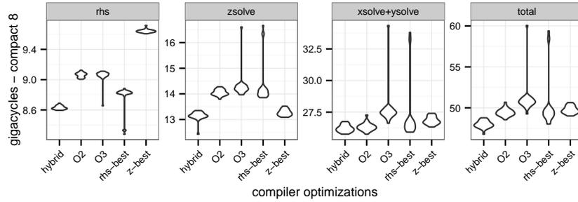
**Fig. 2.** Violin plot execution time of SP regions using best NUMA affinity. Measures were performed 31 times to ensure reproducibility. When measuring total execution time, hybrid compilation outperforms all other optimization levels, since each region uses the best available optimization sequence.
