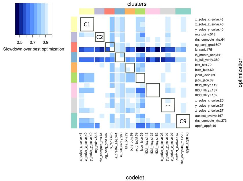
**Fig. 14.** Optimization sequence evaluation across clusters of similar codelets. To build the color matrix, we apply to each codelet (horizontal axis) the best optimization sequence for every other codelet (vertical axis). The color of each cell represents the slowdown over the best sequence found. The square C1 represents the compilation passes of the first cluster applied to the regions within C1.
