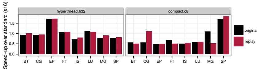
**Fig. 11.** Original and CERE predicted speedup for two thread configurations. Replay speedup is the ratio between the replayed target and the replayed standard configuration. CERE accurately predicts the best thread affinities in six out of eight benchmarks. For CG and MG, we miss-predict configurations that use all the physical cores.
